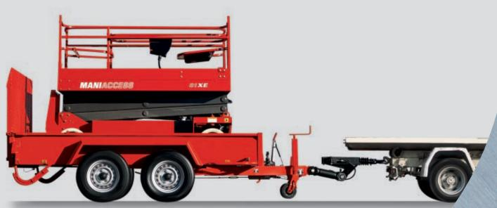
These very light machines can be transported easily on trailers with a maximum weight of 3.5 t.
