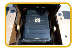
Adopt large-capacity and high-energy density LFP battery which ensure long working time as more than 8 hours after full charged. The battery can be recharged more than 4000 circles and can be used for more than 8 years.
